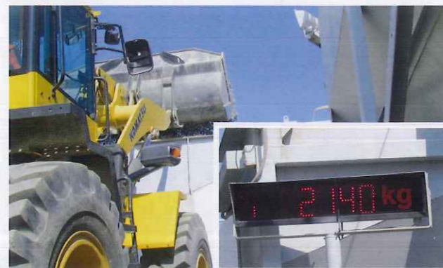
Aggregates are loaded to a high degree of accuracy to displayed amounts
