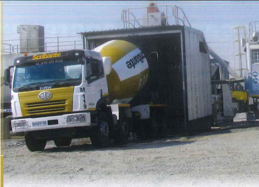
Scribante's mobile batching plant near Fourways, Johannesburg
